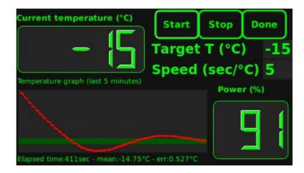
The **Cooling control** tool provides means to control and monitor the CCD temperature during the cooling process and regulation.
