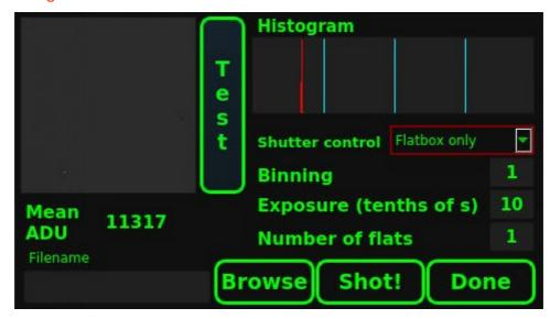
The **Flat maker** tool can be used to check the flats exposure and, once the mean ADU value is the desired one, to create a sequence of flats. The user has to insert the flat **exposure** in tenth of seconds, the **binning** value and select the **shutter control**. There are 3 types of shutter control:
