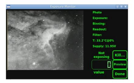
The **Monitor** tool can be used to follow or interrupt the photo sequence currently in progress. It provides the following information related to the current exposure:
