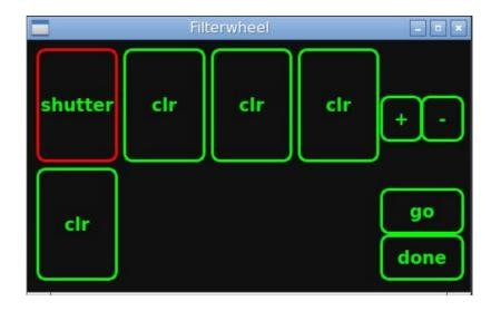
The Filterwheel tool is used to control the integrated filter wheel, to select a filter for the Find and focus and flat maker tools.
